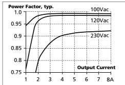
Dec. 2014 / Rev. 2.2 DS-QS10.DNET-EN All parameters are specified at 24V, 8A, 230Vac, 25°C ambient and after a 5 minutes run-in time unless otherwise noted.
