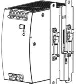
Side mounting with DIN-rail brackets
