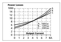
Fig. 9-4 Losses vs. input voltage at 24V, 8A, typ.
