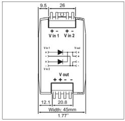
Fig. 14-2 Side view Depth: 91mm, 3.58' └ DIN-Rail depth
