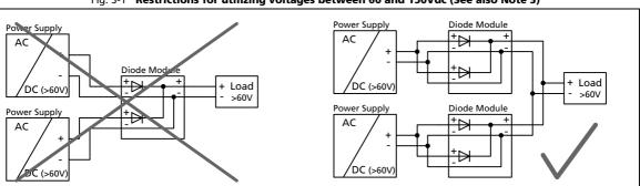
Fig. 3-1 Restrictions for utilizing voltages between 60 and 150Vdc (See also Note 3)
