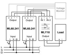
**Please note:** This simple way to build a redundant system does not cover failures such as an internal short circuit in the secondary side of the power
