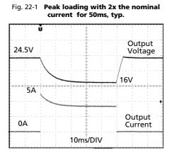
Peak load 5A (resistive load) for 50ms Output voltage dips from 24V to 16V.
