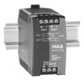
The MLY10.241 is a dual redundancy module, which has two diodes with a common cathode included. It can be used for various purposes. The most popular application is to configure highly reliable and true redundant power supply systems. Another interesting application is the separation of sensitive loads from non-sensitive loads. This avoids the distortion of the power quality for the sensitive loads which can cause controller failures.
