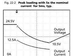
Peak load 12.5A (resistive load) for 5ms Output voltage dips from 24V to 10.5V.
