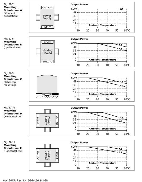
All parameters are specified at 24V, 2.5A, 230Vac 50Hz input, 25°C ambient and after a 5 minutes run-in time unless otherwise noted.
