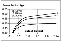
All parameters are specified at 24V, 2.5A, 230Vac 50Hz input, 25°C ambient and after a 5 minutes run-in time unless otherwise noted.
