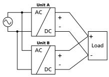
A fuse or diode on the output of each unit is only required if more than three units are connected in parallel. If a fuse (or circuit breaker) is used, choose one with approximately 150% of the rated output current of one power supply.
