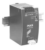
or extends the hold-up time after turn-off of the AC power. In times when the power supply provides sufficient voltages, the buffer unit stores energy in integrated electrolytic capacitors. In case of mains voltage fault, this energy is released again in a regulated process. One buffer module can deliver 20A additional current.
