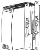
Side mounting with DIN-rail brackets
