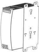
Side mounting without DIN-rail brackets
