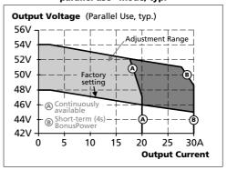
Fig. 6-4 Dynamic overcurrent capability, typ.
