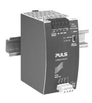
This buffer unit is a supplementary device for DC 48V power supplies. It delivers power to bridge typical mains failures or extends the hold-up time after turn-off of the AC power. In times when the power supply provides sufficient voltages, the buffer unit stores energy in integrated electrolytic capacitors. In case of mains voltage fault, this energy is released again in a regulated process.
