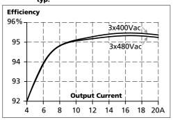
Fig. 11-3 Efficiency vs. input voltage at 48V, 20A, typ.
