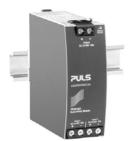
The YR40.482 is equipped with two input channels (20A each), which are individually decoupled by utilizing mosfet technology. The output current can go as high as 40A.
