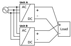
If more than three units are connected in parallel, a fuse or circuit breaker with a rating of 30A or 32A is required on each output. Alternatively, a diode or redundancy module can also be utilized.
