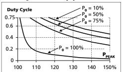
$$DutyCycle = \frac{T_{peak}}{T_{peak} + T_0}$$
