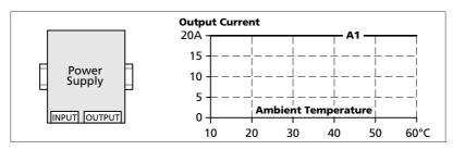
Fig. 24-11 Mounting Orientation B (Upside down)
