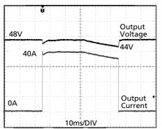
40A Peak load (resistive) for 50ms Output voltage dips from 48V to 44V.
