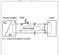
Maximal wire length\*) for a fast (magnetic) tripping:
