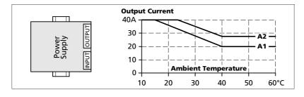
Nov. 2013 / Rev. 3.1 DS-QS40.244-EN All parameters are specified at 24V, 40A, 230Vac, 25°C ambient and after a 5 minutes run-in time unless otherwise noted.
