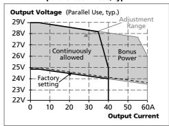
Fig. 6-4 **Dynamic overcurrent capability, typ.**
