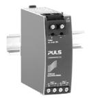
The YR80.242 is equipped with two input channels (40A each), which are individually decoupled by utilizing mosfet technology. The output current can go as high as 80A. Using mosfets instead of diodes reduces the heat generation and the voltage drop between input and output. The YR80.242 does not require an additional auxiliary voltage and is self-powered even in case of a short circuit across the output.
