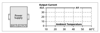
Fig. 25-7 Mounting Orientation B (Upside down)
