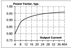
Nov. 2013 / Rev. 3.1 DS-QS40.244-EN All parameters are specified at 24V, 40A, 230Vac, 25°C ambient and after a 5 minutes run-in time unless otherwise noted.
