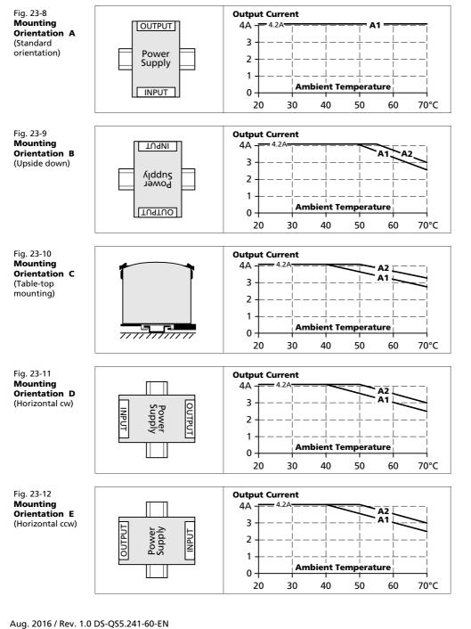
All parameters are specified at 24V, 4.2A, 110Vdc, 25°C ambient and after a 5 minutes run-in time unless otherwise noted.
