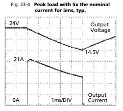
21A Peak load (resistive) for 5ms Output voltage dips from 24V to 14.5V.
