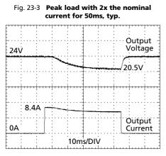
8.4A Peak load (resistive) for 50ms Output voltage dips from 24V to 20.5V.
