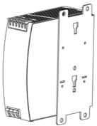
Side mounting with DIN-rail brackets
