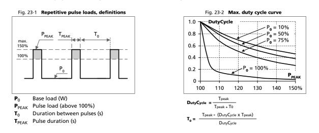
**Example:** A load is powered continuously with 100W (= 50% of the rated output load). From time to time a peak power of 300W (= 150% of the rated output load) is needed for 1 second.
