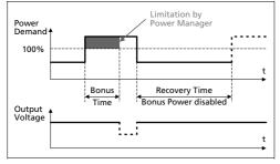
The BonusPower<sup>®</sup> is available as soon as power comes on and immediately after the end of an output short circuit or output overload.
