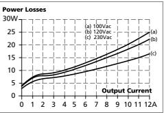
Fig. 9-4 Losses vs. input voltage at 10A, typ.
