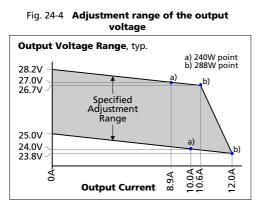
The output voltage shall only be changed when absolutely necessary, e.g. for battery charging as described in the next chapter.
