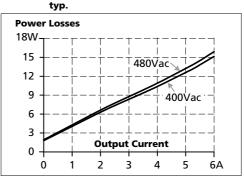
Fig. 8-4 Losses vs. input voltage at 24V, 5A, typ.
