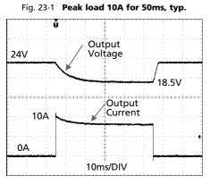
Peak load 10A (resistive load) for 50ms Output voltage dips from 24V to 18.5V.
