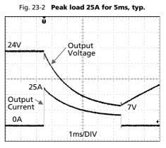
Peak load 25A (resistive load) for 5ms Output voltage dips from 24V to 7V.
