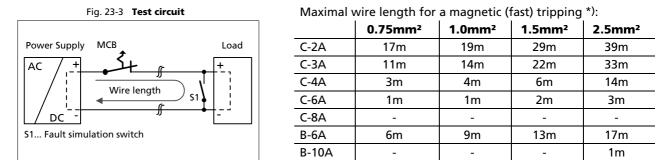
\*) Don't forget to consider two times the distance to the load (or cable length) when calculating the total wire length (+ and - wire).
