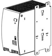
Side mounting without DIN-rail brackets
