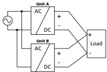
If more than three units are connected in parallel, a fuse or circuit breaker with a rating of 30A or 32A is required on each output. Alternatively, a diode or redundancy module can also be utilized.
