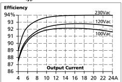
Fig. 9-3 Efficiency vs. input voltage at 24V, 20A. tvp.
