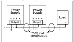
Fig. 12-2 Using distribution terminals
