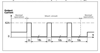
Fig. 6-4 Dynamic overcurrent capability, typ.
