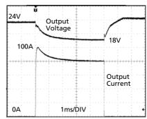
100A Peak load (resistive) for 5ms Output voltage dips from 24V to 18V.
