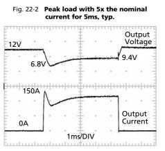
150A Peak load (resistive) for 5ms Output voltage dips from 12V to 9.4V.
