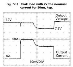
60A Peak load (resistive) for 50ms Output voltage dips from 12V to 7.8V.
