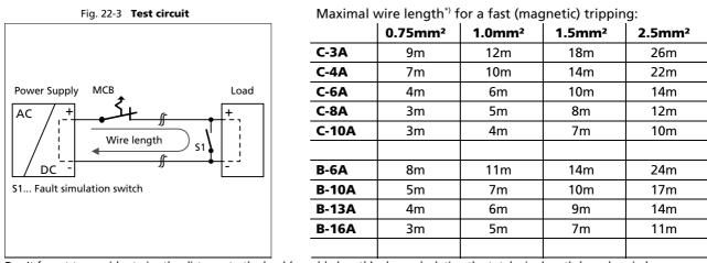
\*) Don't forget to consider twice the distance to the load (or cable length) when calculating the total wire length (+ and - wire).
