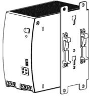
Side mounting with DIN-rail brackets
