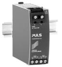
The YR80.242 is the preferred redundancy module for the CPS20.121 power supply. It is equipped with two input channels, which are individually decoupled by utilizing mosfet technology. Using mosfets instead of diodes reduces the heat generation and the voltage drop between input and output. The YR80.242 does not require an additional auxiliary voltage and is self- powered even in case of a short circuit across the output.
