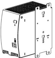
Side mounting without DIN-rail brackets
