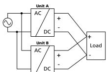
If more than three units are connected in parallel, a fuse or circuit breaker with a rating of 40A or 50A is required on each output. Alternatively, a diode or redundancy module can also be utilized.
