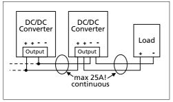
Fig. 12-2 Using distribution terminals
