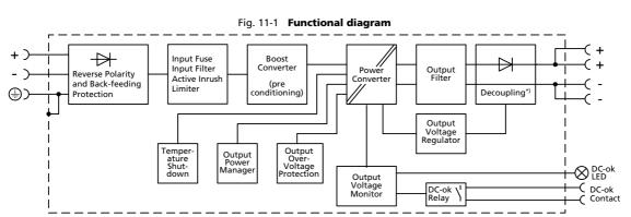
Decoupling: This feature utilizes a Mosfet instead of a diode in order to minimize the voltage drop and power losses.
