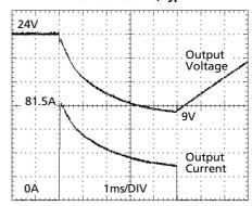
81.5A Peak load (resistive) for 5ms Output voltage dips from 24.5V to 9V.
