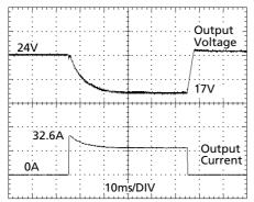
32.6A Peak load (resistive) for 50ms Output voltage dips from 24.5V to 17V.
