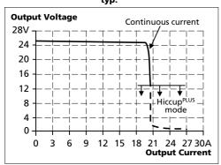
Fig. 6-2 Short-circuit on output, Hiccup<sup>PLUS</sup> mode, typ.
