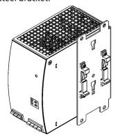
Side mounting with DIN-rail brackets
