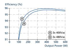
Fig. 9-1: Efficiency vs. output current at 24V, typ.
