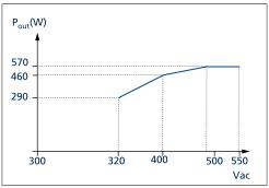
Fig. 23-1: Two phase power capability
