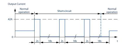
Fig. 6-2: Short-circuit on output, Hiccup<sup>PLUS</sup> mode, typ.
