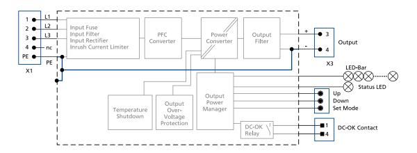
Fig. 12-1: Functional Diagram FPT500.241-002-101
