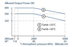
Fig. 16-2: Output power vs. ambient temp.
