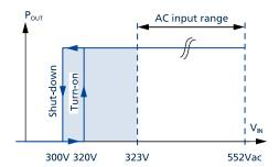
Fig. 3-1: Input voltage range
