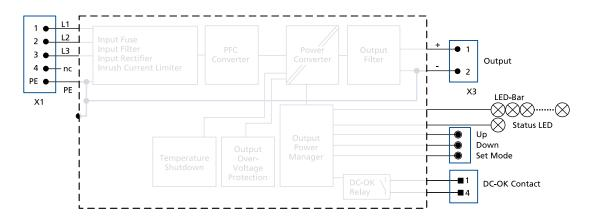
Fig. 12-3: Functional Diagram FPT500.241-010-108
