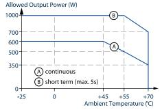
Fig. 16-1: Output power vs. ambient temp.
