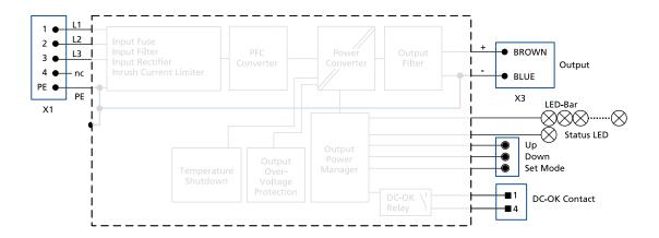
Fig. 12-2: Functional Diagram FPT500.241-006-104
