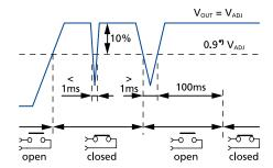
Fig. 8-1: DC-OK relay contact behavior
