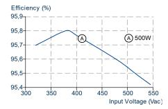
Fig. 9-3: Efficiency vs. input voltage at 24V, 500W, typ.
