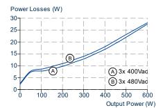
Fig. 9-2: Losses vs. output power at 24V, typ.
